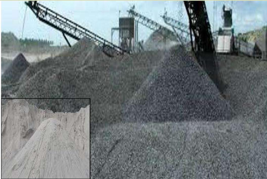
M-sand is *Manufactured Sand* by crushing granite rocks into crystalline powder which is becoming an alternative to river sand for construction purposes. This has been a practice nowadays for its ease-of-availability while the “real” sand is depleting fastly. Despite known for its cheaper cost, M-sand is not so nearer to the real one when it comes to durability and strength. The use of M-Sand symbolizes how much the human activity in the last few decades have exhausted the natural resources.
