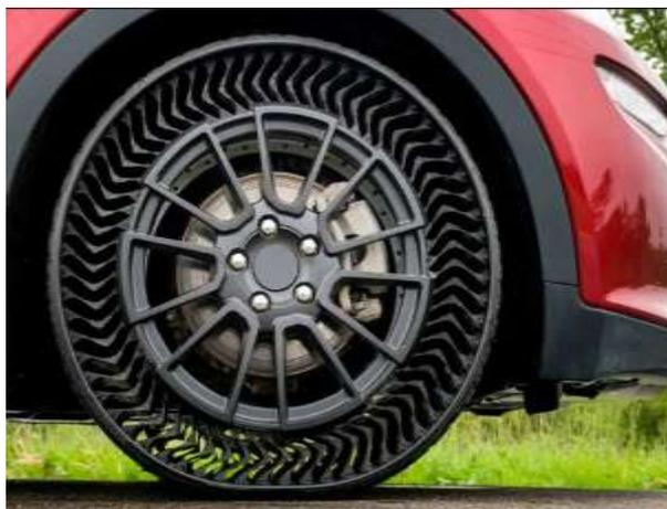
Michelin has been working at making airless tyres for the past five years now. The company showcased the Tweel concept in 2014 and an investment of \$50 million has gone into the new plant for making it ready for commercial usage. The Uptis is a version of this and is airless. It completely eliminates the risk of flat tyres and blowouts.
